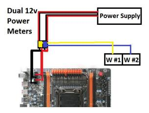
Here is how I measured the power; I used two 12v meters made by Zalman. Each can only measure up to 250Watts, so I modded two of them together, and I add the resulting numbers. Remember that to measure current you need to break the circuit.
