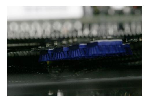
**Fan for the board:** If you are using watercooling then you are disregarding the airflow required around the CPU socket, particularly for the memory and VRM. With SB heat wasn't really the enemy, but with SBe it is the #1 enemy. A fan over the VRM heatsink is recommended for all LGA2011 boards. You will even see Alienware computers come with directional fan over the VRM with LGA2011 boards.
